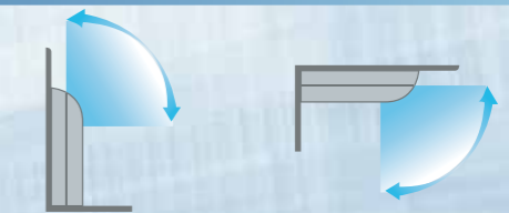
The unit can be installed either horizontally on the ceiling or vertically against the wall.
